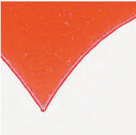
Figure 4: Halo effect at the edges in the form of a light outline around the printed area
