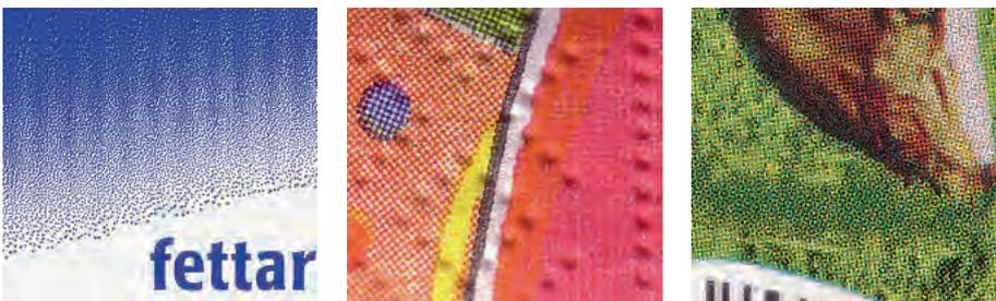
Figure 1: A comparison of different print products: a) simple corrugated board printing, b) napkin printing, c) beverage package
