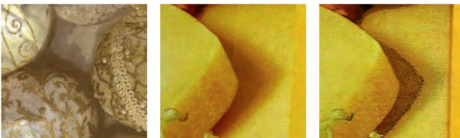
Figure 2: Visible banding in the printed image
