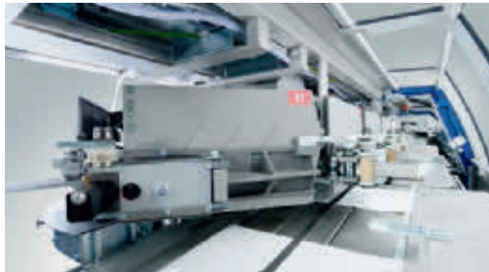
The KM 600.C perfect binder for conventional post-press jobs, targeted at the fast, cost-competitive production of brochures, magazines, catalogues and book blocks.
