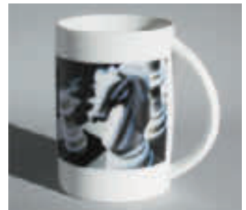
One example for the outstanding results that can be achieved with sheetfed gravure printing. Compared with screen printing, much finer screen rulings can be printed in gravure and therefore image details can be reproduced in a 'photorealistic' way even on porcelain.
