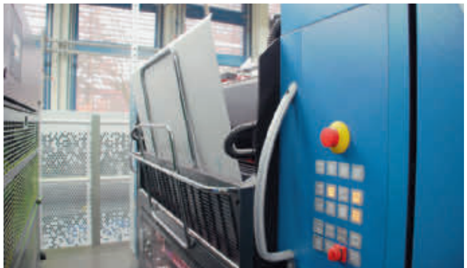
Direct plate cylinder drives enable automatic plate changing (ten units in one minute) and washing processes to run parallel to each other. That takes a significant slice off job changeover times.
