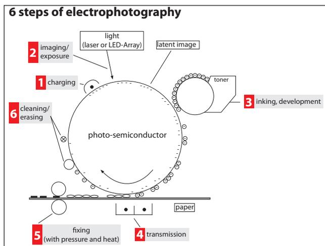
Figure 1: The electrophotographic printing process
