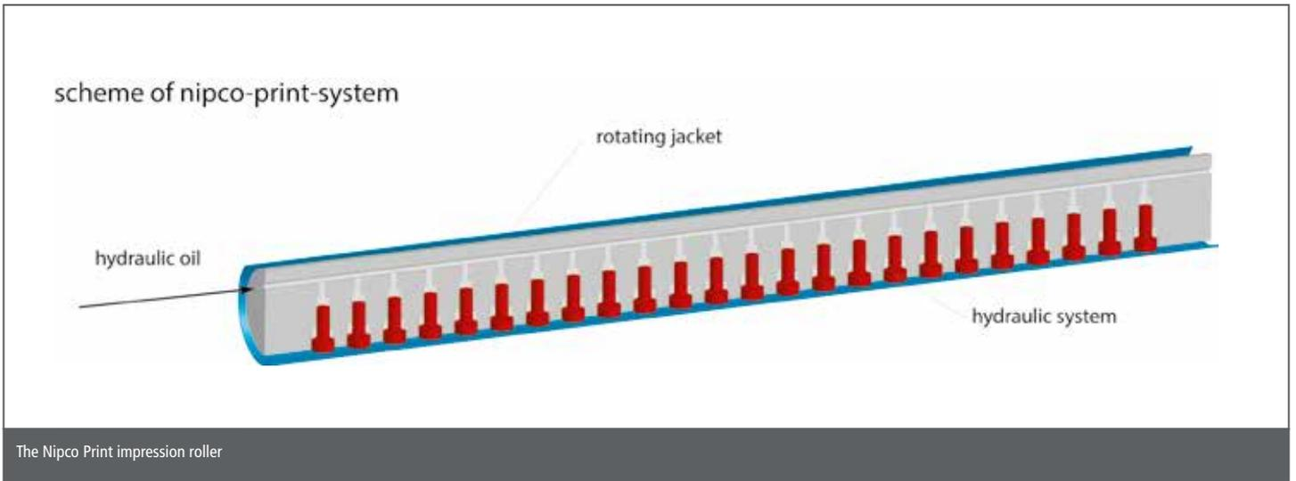
covered by a rotating jacket. In the impression roller core, there are channels through which hydraulic oil is pumped in order to stretch the impression roller jacket towards the gravure cylinder. A similar method is used in the Nipco print impression roller system. It has an impression roller core with a hydraulic system covered by a rotating, elastic jacket. By means of the hydraulic stamps, the impression roller jacket can be pressed towards the gravure cylinder in high precision.
