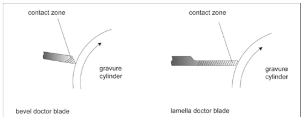
Wedge-shaped, bevelled doctor-blade and lamella doctor-blade
