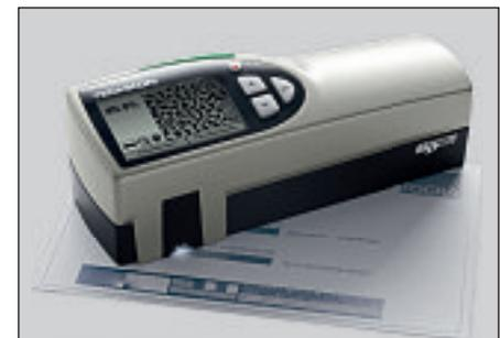
No guarantee of the print quality achieved without control of the printing plate quality. While initially CtP plates were checked with densitometers designed for use on printed sheets, since there were no alternatives, devices based on microscopic image capture and image analysis are overwhelmingly used now.
