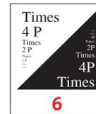
The fourth patch of the graphic (6) shows positive and negative fonts of different size (0.5, 1, 2, and 4 pt). They enable to assess the effects of low resolution of the plate, spot unbalance and/or missing linearity in practical applications.
