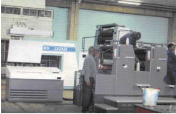
Machine operator checking the plate cylinder of the Speedmaster SM-74 installed at the Government Printing Department.
