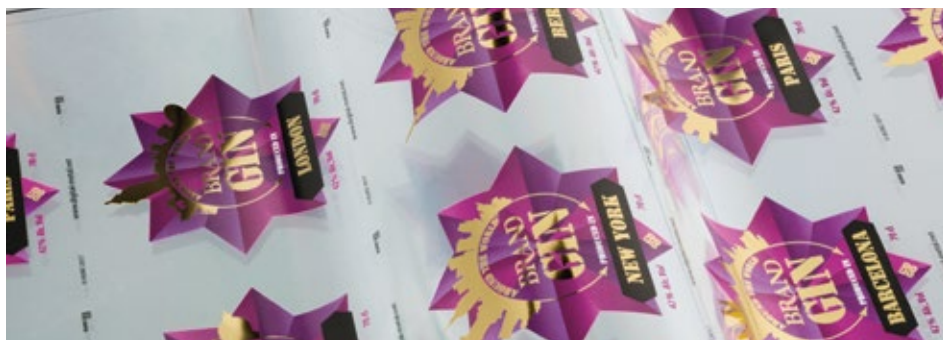
Web-fed labels finished with variable designs using KURZ DM-Liner UV-Ink technology
