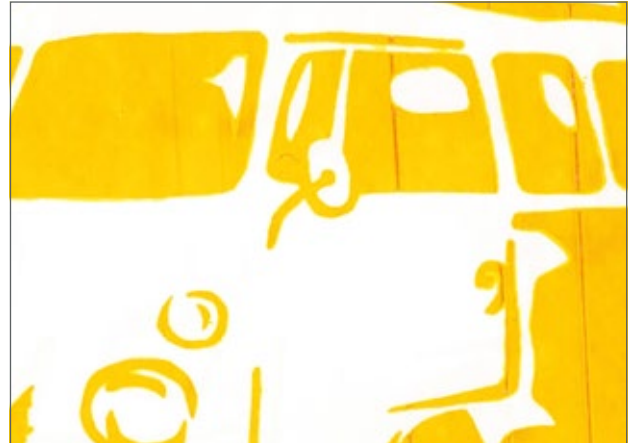
A typical misprint: Streaks in the printed image
