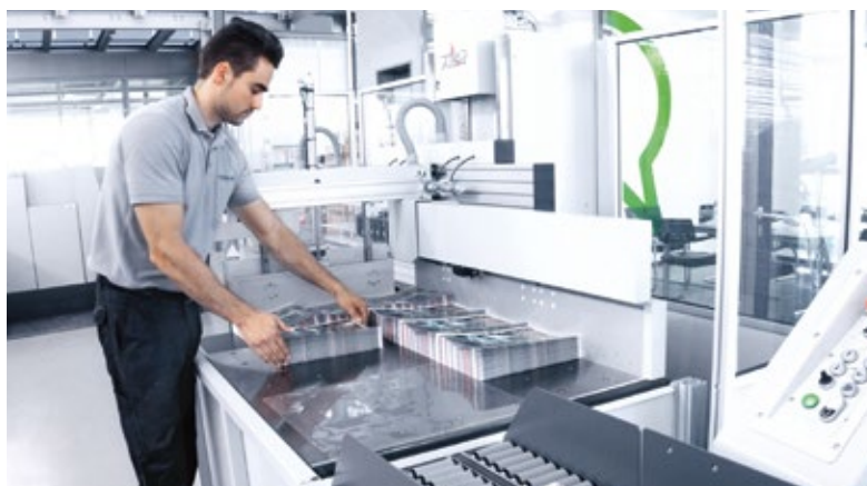
Ergonomic stacking of folded sheets with POLAR Transomat TRE
