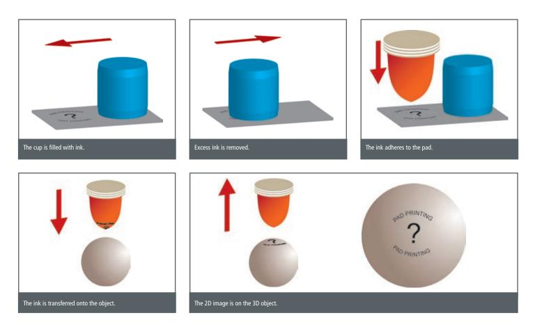
from escaping. For the closed system, an additional "parking zone" must be planned for the doctoring cup in addition to the proper motif surface on the printing plate. Inking of the printing plate is carried out by travelling over the motif area with the doctoring cup. The closed system protects the ink from evaporation of the solvents and contaminations. The doctoring cup remains in the parking zone while the pad takes the ink from the cups and prints. Then this cycle begins again.
