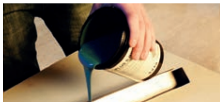
Filling of the coating trough
