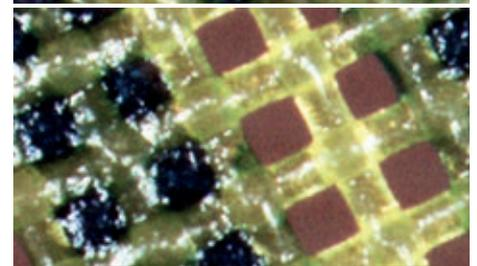
On the top: Fabric with copying layer ready for print. Center and bottom: Details of the copying layer on the mesh.
