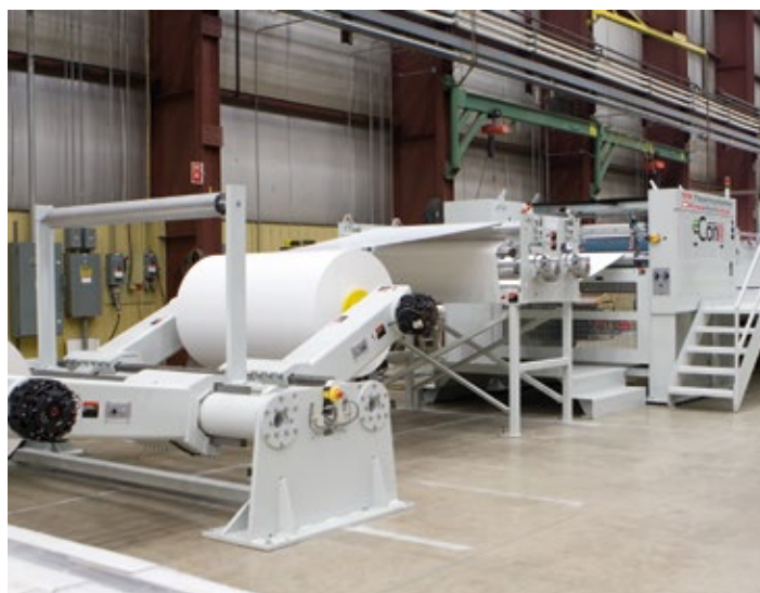
The eCon sheeter from BW Papersystems with its on-machine cross cut knife sharpening offers high sheet cutting quality.
